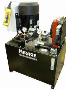
HYPP60-30- 3ph 15 hp tandem hydraulic power pack 50 lpm / 20 lpm @ 70 bar – 380/440v 3 phase – pendant control
