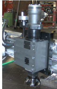
WP6000-8 Extended milling spindle – 250mm stroke
